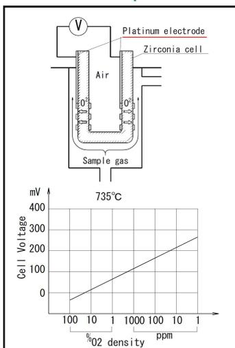
Sensing cell is a closed end, 90mm length and 7mm diameter. Tube made of Zirconium oxide. When it is red hot, it becomes an oxygen measuring cell because of movement of oxygen ions in its crystal structure.
