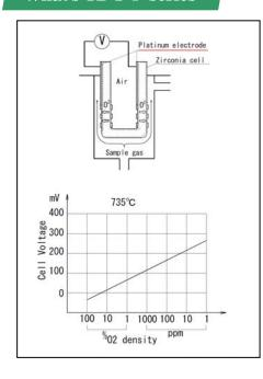
Sensing cell is a closed end, 90mm length and 7mm diameter. Tube made of Zirconium oxide. When it is red hot, it becomes a oxygen measuring cell because of movement of oxygen ions in its crystal structure.
